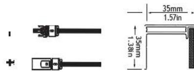
PV Connector Model - TT01, 1000V, 30A, IP67
